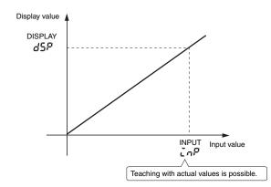
Instead of setting by inputting with the <a> Up Key and <a> Shift Key, current values can be input as scaling input values for teaching. This is useful for making settings while checking the operation status of the K3MA-F.
