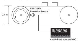
Here, the conveyor belt feed speed is to be displayed in units of 0.1 m/min.
