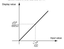
When displaying a flowrate (e.g., in  $\mathscr{U}$ min or  $\mathscr{U}$ h), make the scaling settings after confirming the I/O characteristics of the flowrate sensor. There are flowrate sensors that output analog signals. If this kind of flowrate sensor is used, consider using the K3MA-J.
