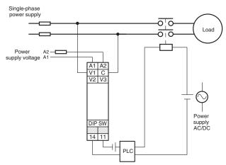
Note: Use copper wires with a rating of 75°C or an equivalent rating.
