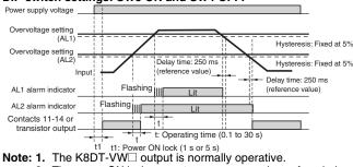
2. The power ON lock prevents unnecessary alarms from being generated during the instable period when the power is first turned on. There is no relay output during timer operation.
