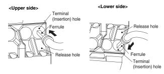
If a wire is difficult to connect because it is too thin, use a flat-blade screwdriver in the same way as when connecting stranded wire.
