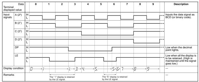
• Using the latch input (LE) terminal for each Unit, the data input terminals (A to D) can be used in common yet still enable display on each Unit (example of a 3-digit dynamic-output model with positive logic).
