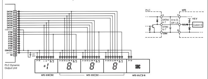
2. Connected to C200H-OD215 Transistor Output Unit \*2 \*3
