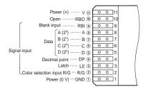
Note: 1. The latch terminal on  $\pm 1$ . Display Units is provided only on Dynamic Output Models.
