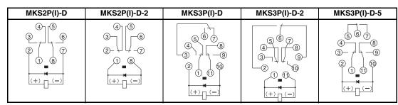
Diode Type (DC Coil: Reverse Polarity)
