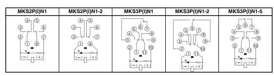
Diode Type (DC Coil: Standard Polarity)
