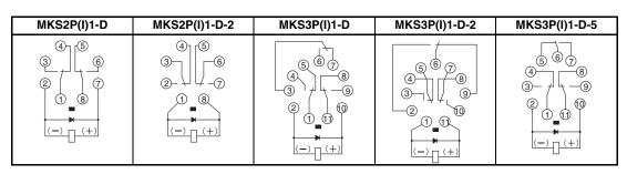
**LED Indicator and** Diode Type (DC Coil)
