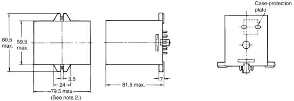
Note 1: As shown in the diagram, there are three 10-dia. holes in the side of the case for MM□XP(N, -D). 2: When a case-protection plate is attached, the width of the Relay will be 80 mm max.
