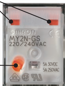
Relay with AC Coil (LED: Red)
