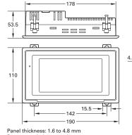
Recommended cut-out size:  $178.5 \, ^{+0.5}/_{-0} \times 100.5 \, ^{+0.5}/_{-0} \text{ mm (W x H)}$
