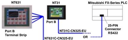
The FX0 and FX0N PLCs use a different connector than the other FX series PLCs. Connect the Omron cable to the FX-20P-CADP cable from Mitsubishi, then connect it to the PLC communication port.
