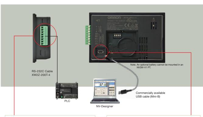
Serial Communications/Power Supply Connector
