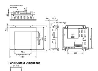
Applicable panel thickness : 1.6 mm to 4.8 mm
