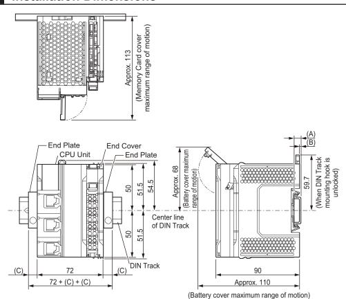
W: Width of CPU Unit (including the End Cover)
