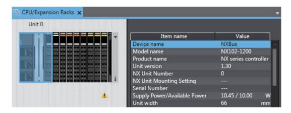
The Sysmac Studio does not consider the I/O power supply design conditions. When actually designing the power supply, refer to 4-3-2 Designing the I/O Power Supply from the NX Bus on page 4-14.
