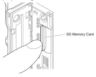
The SD Memory Card will be ejected from the compartment.
