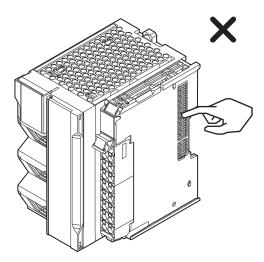
Do not write on the CPU Unit with ink within the restricted region that is shown in the following figure. Also do not get this area dirty. When the Unit is installed or removed, ink or dirt may adhere to the pins in the NX bus connector, which may result in malfunctions in the Unit.
