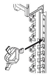
**2** Rotate the runner to break off the Coding Pin.
