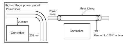
Example: Separating Controller from Power Lines
