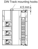
DIN Track Mounting Hooks in Locked Position
