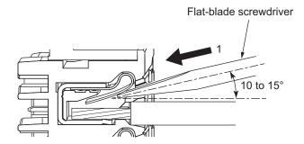
**2** Leave the flat-blade screwdriver pressed into the release hole and pull out the wire.
