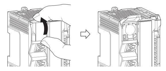
3 Connect the connector of the battery to the battery connector and insert the battery in the battery slot.
