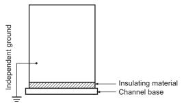
Example: Insulating and Grounding an Enclosure
