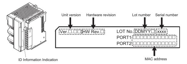
Note The hardware revision is not displayed for the Unit that the hardware revision is in blank.
