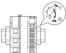
To remove an End Plate 1) insert the tip of a flat-blade screwdriver into groove "a" and 2) use "b" as a fulcrum and lift the end of the screwdriver, as shown in the following diagram.
