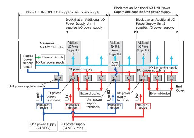
However, fewer protective devices may be required when the current consumption of each block does not exceed the rated current.
