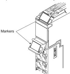
The marker attachment locations on the NX Units depend on the type of external connection terminals. Refer to the user's manual for the NX Units that you will use for the marker attachment locations.
