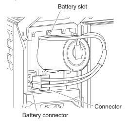
**4** Press in the battery harness by twisting and attach the battery cover.
