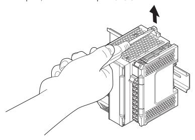
Remove the CPU Unit from the DIN Track.
