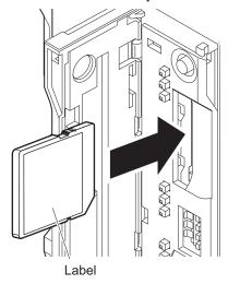
**3** Push the SD Memory Card securely into the compartment.
