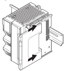
**2** Press the End Cover firmly against the DIN Track until you hear it lock into place on the DIN Track.
