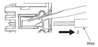
**3** Remove the flat-blade screwdriver from the release hole.
