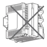
Mounting with the DIN Track Installed Vertically
