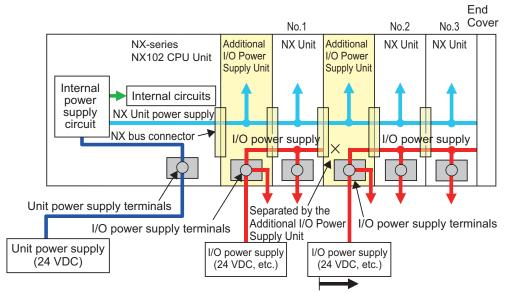
When the I/O power supply becomes the following states for the subsequent NX Units.
