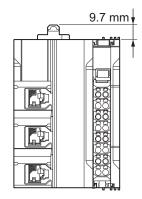
DIN Track Mounting Hooks in Unlocked Position
