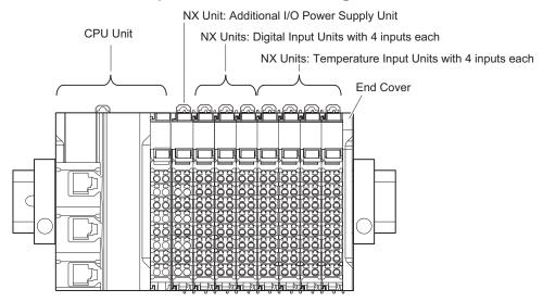
The widths of the Units in the example CPU Rack configuration and the total configuration width are given below.
