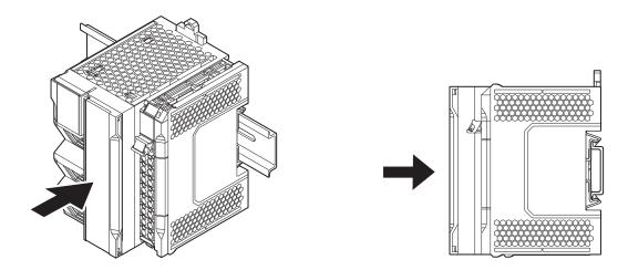
Press the DIN Track mounting hooks down to the locked position.
