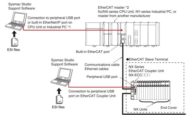
\*1. The connection method for the Sysmac Studio depends on the model of the CPU Unit or Industrial PC.
