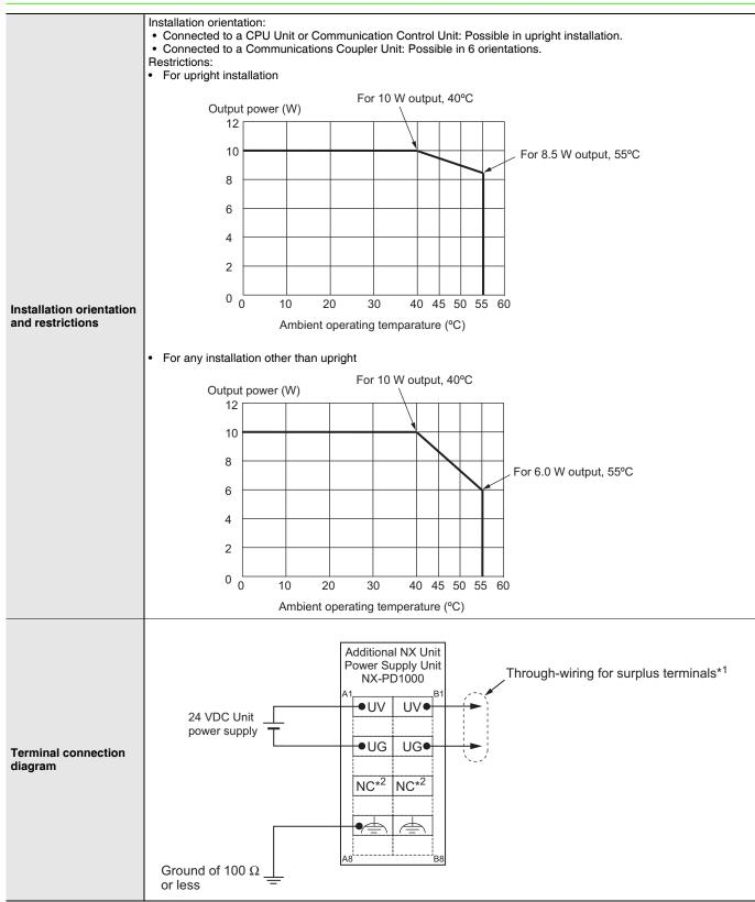
\*1. You can use the unwired terminals of the Unit power supply terminals (UV/UG) for through-wiring of the Additional NX Unit Power Supply Unit or the Unit power supply terminals on the EtherCAT Coupler Unit.
