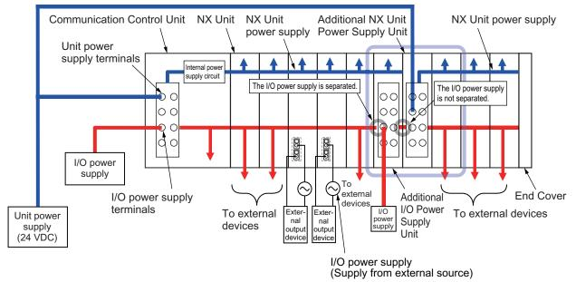
Note: Supply the Unit power and the I/O power from different power supplies. If you supply power from the same power supply the galvanic separation between the bus system and the I/O circuits is no longer effective. Noise generated in the I/O circuits may cause malfunctions in the internal circuits of the units.
