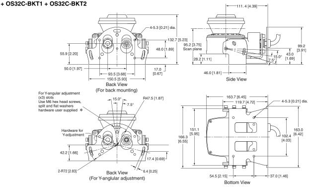
\* In order to comply with Section 4.2.16 of IEC 61496-3, when the OS32C is mounted where the scanner position could change (e.g. as the result of an impact), additional mechanical means, such as serrated or toothed lock washers, must be employed in the mounting hardware.
