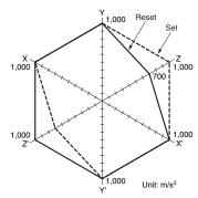
Sample: G6BK-1114P-US Number of Relays: 12 pcs Test Conditions: The value at which malfunction occurred was measured after
