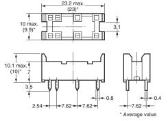
PCB Mounting Holes (BOTTOM VIEW)
