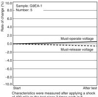
Characteristics were measured after applying a shock of 490 m<sup>2</sup>/s to the test piece 3 times each in 6 directions along 3 axes. The percentage rate of change is the average value for all of the samples.
