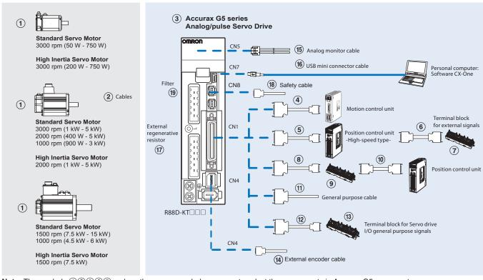
Note: The symbols (12345)... show the recommended sequence to select the components in Accurax G5 servo system
