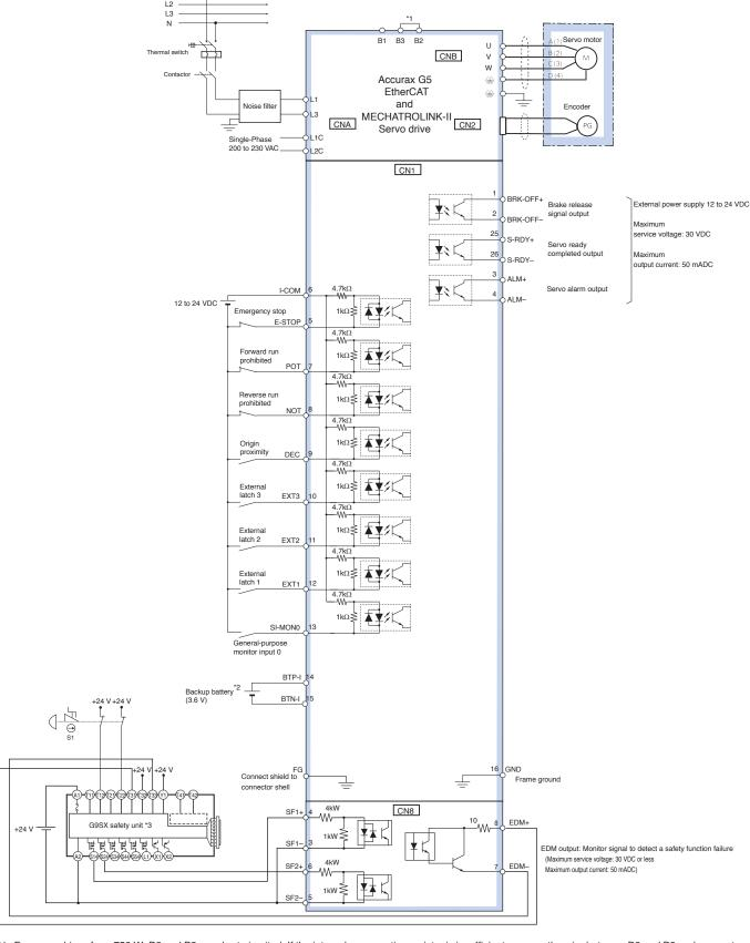
For servo drives from 750 W, B2 and B3 are short-circuited. If the internal regenerative resistor is insufficient, remove the wire between B2 and B3 and connect an external regenerative resistor between B1 and B2.
