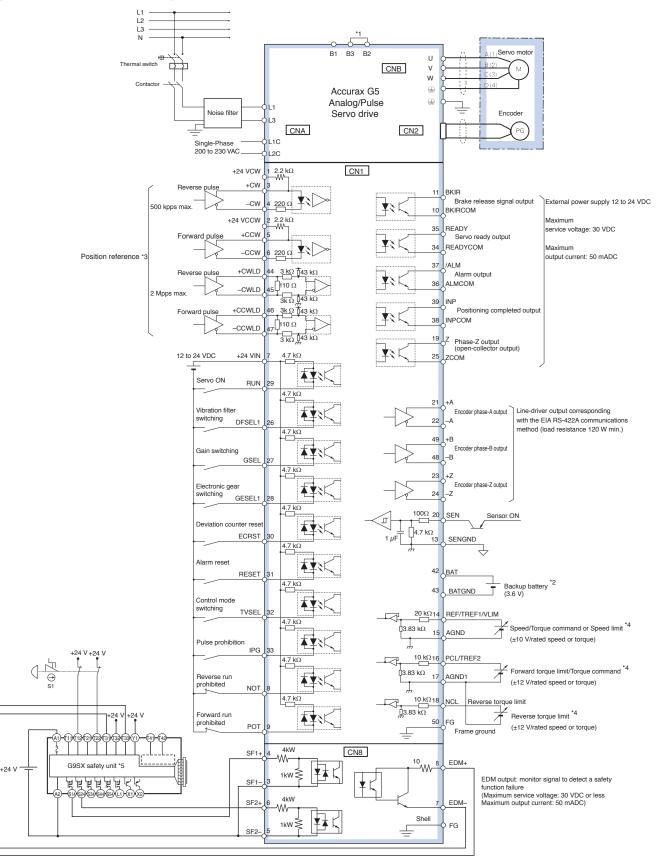
For servo drives from 750 W, B2 and B3 are short-circuited. If the internal regenerative resistor is insufficient, remove the wire between B2 and B3 and connect an \*1 external regenerative resistor between B1 and B2.
