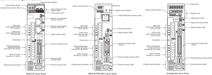
Note: The above pictures show 230 V servo drives models only. The 400 V servo drives have 24 VDC power input terminals for control circuit instead of L1C and L2C terminals.
