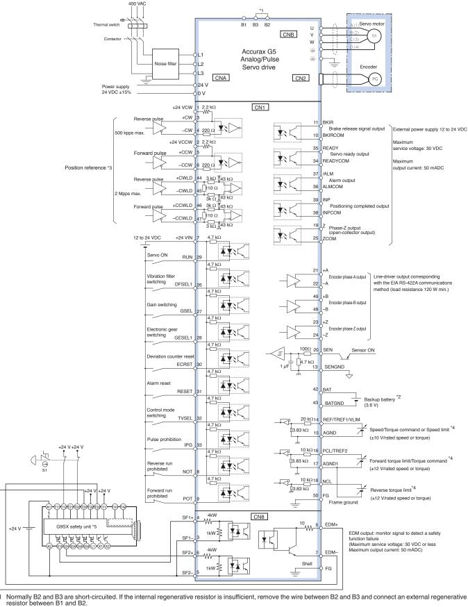
Note: The input function of pins 8,9 and 26 to 33, and output function of pins 10, 11, 34, 35, 38 and 39, can be changed via parameter settings.
