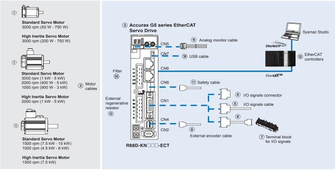
Note: The symbols 12345... show the recommended sequence to select the components in Accurax G5 servo system
