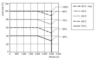
Note: At a voltage below 100 VDC, reduce the load by multiplying with the coefficient 0.9.
