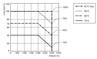
Note: At a voltage below 100 VAC, reduce the load at the rate of 1.3%/V.
