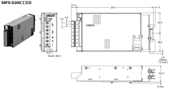
Note: Use a Front-mounting Bracket (S82Y-FSG-30F) when the DIN Rail is not strong enough for your usage environment.
