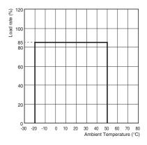
Note: At a voltage below 100 VAC, reduce the load at the rate of 1.3%/V.
