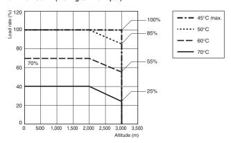
**Note:** At a voltage below 100 VAC, reduce the load at the rate of 1.3%/V. ( $40^{\circ}C$  < Ambient temperature  $\leq 70^{\circ}C$ )
