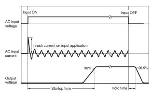
Note: The total inrush current of all of the Power Supplies will flow for parallel operation or backup operation.
