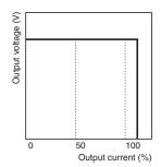
Note: 1. Internal parts may occasionally deteriorate or be damaged if a short-circuited or overcurrent state continues during operation
