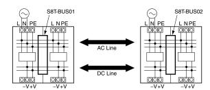
Figure 1: DC line connected (parallel connection)
