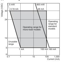
The above diagram is for standard conditions (+5°C to +35°C, 40% to 70%RH). Since the values vary depending on the operating environment conditions, contact your OMRON representative for further details.
