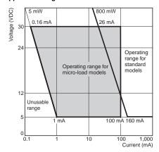
The above diagram is for standard conditions ( $+5^{\circ}C$  to  $+35^{\circ}C$ , 40% to 70%RH). Since the values vary depending on the operating environment conditions, contact your OMRON representative for further details.
