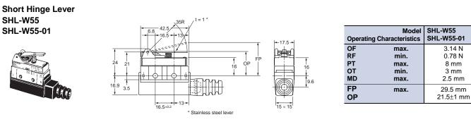
Note: Unless otherwise specified, a tolerance of  $\pm 0.4$  mm applies to all dimensions.
