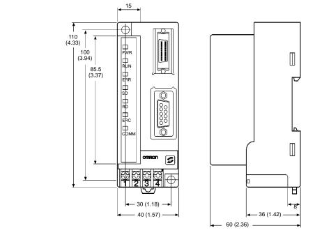
The above dimensions apply to the SRM1-C02-V2. The SRM1-C01-V2 has no RS-232C port.
