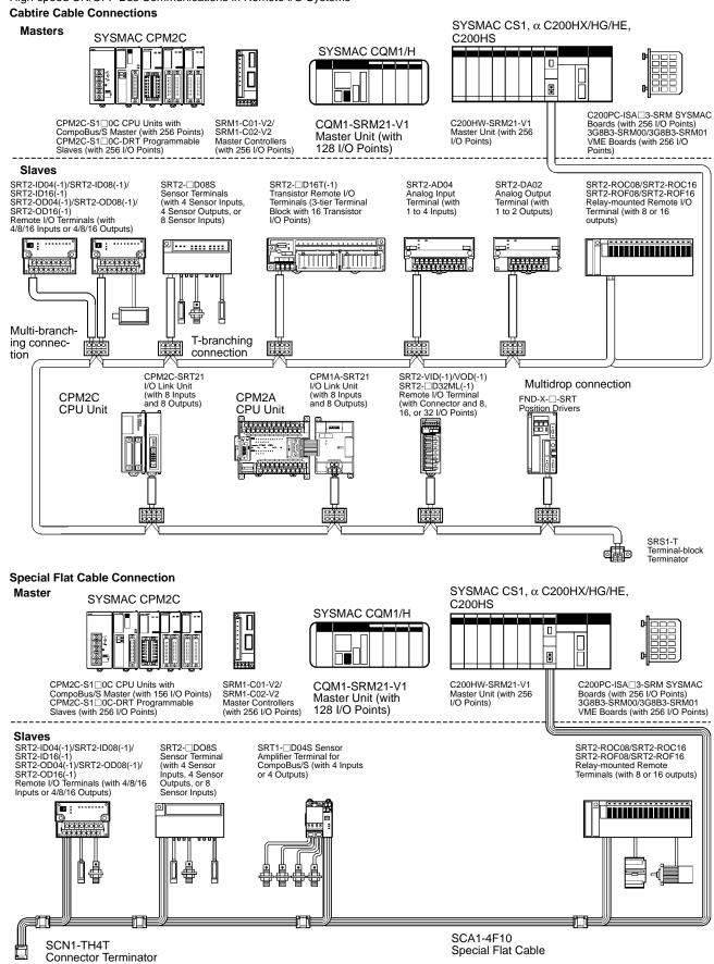
Note: Cabtire cable and flat cable cannot be used together.
