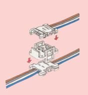
Flat cable can be used with T-branch connectors which allow an increase in the number of Slaves.
