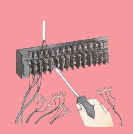
Repeater terminal blocks must be added and wired for I/O expansion.
