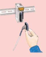
CompoBus/S connector models allow snap-on attachment.
