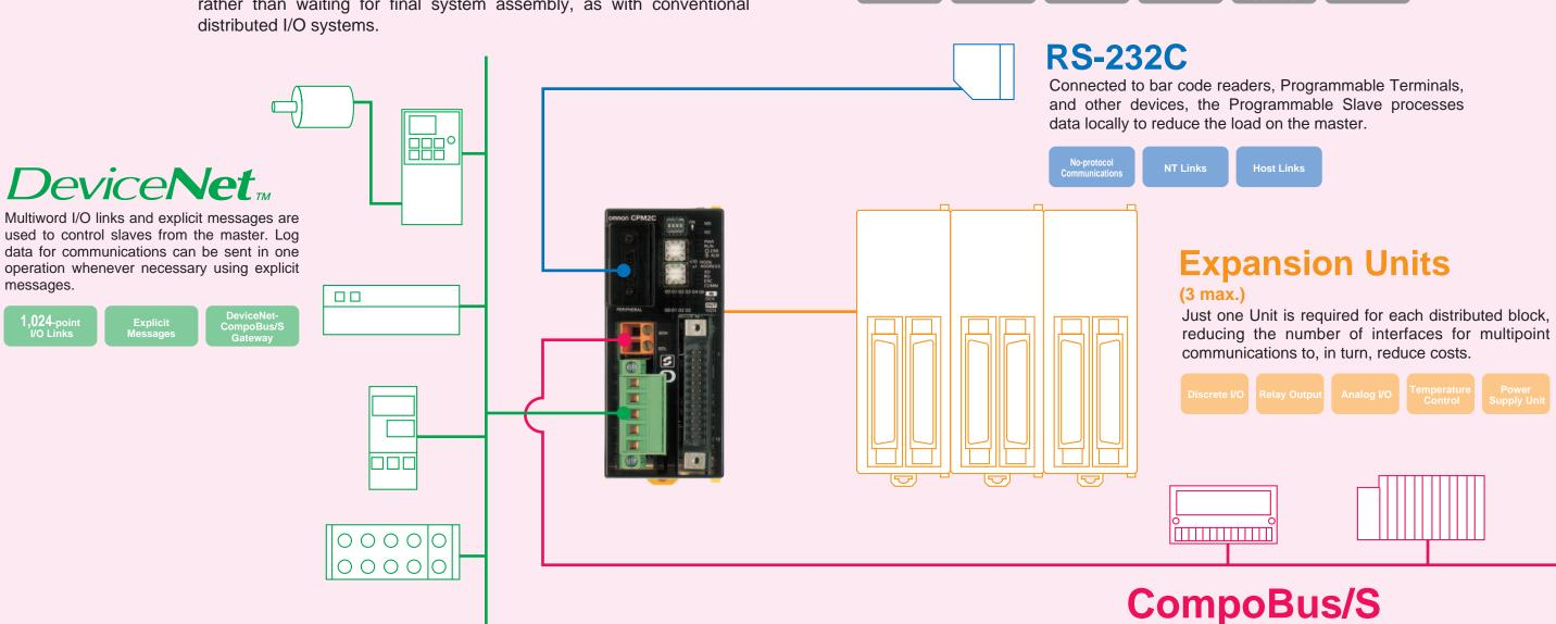
Less wiring is required for terminal block expansions, connections to remote devices (such as signal lights or pushbutton switches), and connections to pneumatic valves and other non-OMRON products.
