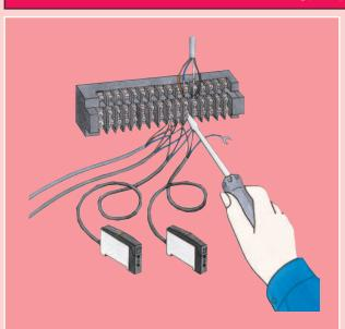
Individual wires must be replaced when using repeater terminal blocks.
