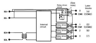
**Note:** The G3DZ-2R6PL Power MOS FET Relay is inserted into this portion of the SRT2-R0F08 and SRT2-R0F16.
