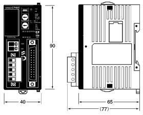
Note: Refer to CPM2C-S Programmable Controller Operation Manual (W377) for detailed specifications.
