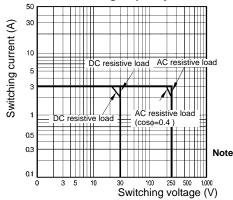
These graphs show the characteristics for when the SRT2-ROC□□ or B1T-JR model is mounted.
