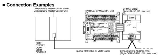
Note: A single CompoBus/S I/O Link Unit together with a maximum of two other Expansion I/O Units can be connected to the CPM1A or CPM2A CPU Unit.
