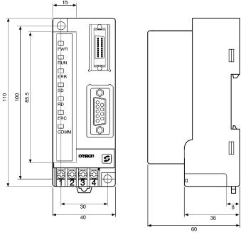
The above dimensions apply to the SRM1-C02-V2. The SRM1-C01-V2 has no RS-232C port.
