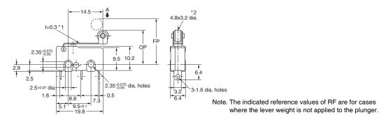
\*1. Stainless-steel lever \*2. Polyacetal resin roller
