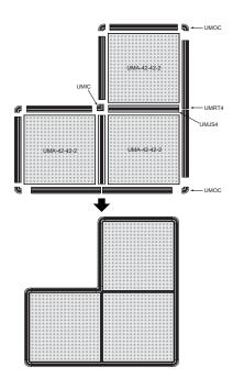
In this case, the perimeter of the Safety Mat is about 84 in., the joint between the Safety Mats is 84 in. long, and the following pieces are required:
