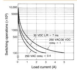
Reference: A maximum current of 0.15 A can be switched at 125 VDC ( $\cos\phi = 1$ ). Maximum current of 0.1 A can be switched if L/R is 7 ms. In both cases, a life of 100,000 operations can be expected. The minimum applicable load is 10 mA at 5 VDC (failure level: P).
