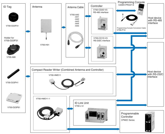
Note: The V700-CD1D-V3, V700-HMD11(-1), and V700-L12 all have different function and command structures.
