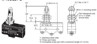
Note: Do not use both the M12 mounting screw and the mounting holes in the case at the same time. Doing so will cause stress to be applied to the Switch, possibly damaging the case or cover.
