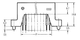
XC5K DIP terminal cross-section diagram
