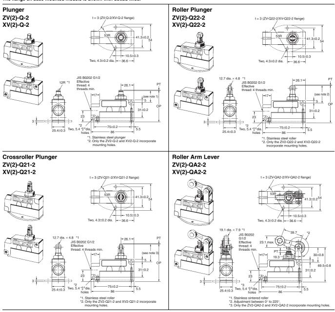
Note: Unless otherwise specified, a tolerance of  $\pm 0.4$  mm applies to all dimensions.
