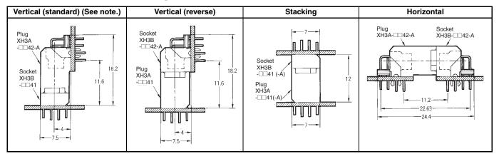
Note: The function of the standard and reverse models is the same as that of the standard XC5 DIN Connectors.
