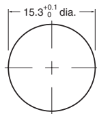
Panel Cutout Dimension Panel thickness = 1 to 4 mm
