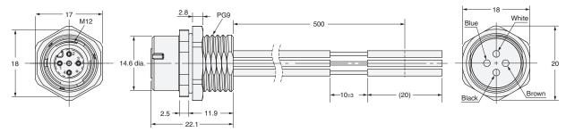
XS5P-D427-5 Rear Panel-mounting Sockets for Front Lock Nuts
