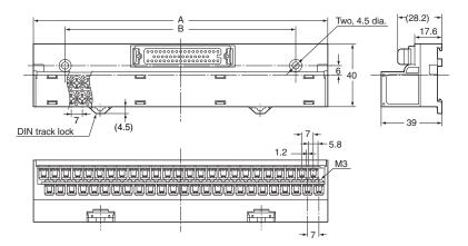
Note: There is only one DIN Track lock located in the center of the Connector for a 20-pole Unit.
