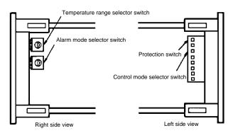
Select the desired temperature range by using the temperature range selector switch (rotary DIP type). The other rotary DIP switch is used to select one of eight alarm functions. Be sure the set temperature and alarm values are within the new range. Otherwise, the temperature controller automatically shifts these values to the maximum or minimum of the newly-set temperature range.
