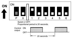
When a quick response in required, set switch 2 to ON to select a proportional period of 2 seconds. Even when a solid state relay (SSR) is used, set the 2-second proportional period only when quick response is essential. Avoid using this setting with a contact output because it will shorten the relay's service life.
