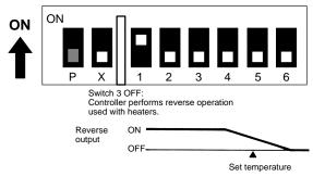
By contrast, if the temperature controller is used to control a cooling device such as a chiller or freezer, set switch 3 to ON.
