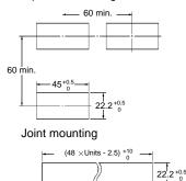
Waterproofing is not possible for joint mounting
