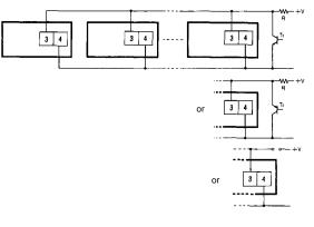
Note: H (Reset ON) level must be 4.5 V minimum.  $H = \frac{4.7 (k\Omega)/N + V}{100}$
