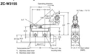
Note: 1. Unless otherwise specified, a tolerance of  $\pm 0.4$  mm applies to all dimensions. 2. Operating characteristics are for when the Switch is operated from direction A.
