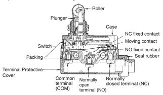
Note: M4 binding head screws (with toothed washers) are used as the terminal screws.
