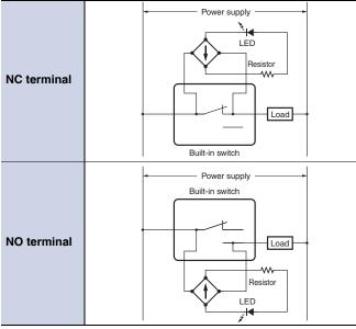
Note: If the wiring is as shown above, the operation of the respective parts will be as shown in the following table. The LED terminals are not wired when the Switch is delivered. Connect it as required.
