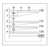
PLCs execute ladder programs one rung (circuit) at a time, starting with the top rung and executing it in order from the left. When the END instruction is reached, the program is executed again from the first rung.
