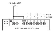
Note: When connected to the positive (+) common, I4 and I5 cannot be used as analog inputs.
