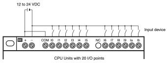
Note: When connected to the positive (+) common, la and lb cannot be used as analog inputs.
