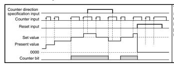
The counter bit turns ON when the counter value (present value) reaches the set value (present value  $\geq$  set value). The counter returns to 0 and the counter bit turns OFF when the reset input turns ON. Count inputs are not accepted while the reset input is turned ON. The counter present value and counter bit (ON/OFF) are held even if the operating mode is changed or the power supply is interrupted.
