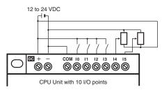
Note: When connecting an analog input device, always connect the negative side to the COM terminal.
