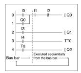
ZEN executes the entire ladder program (up to 96 lines) from the first to last line at one time. Each row is executed in order from left to right starting from the left bus
