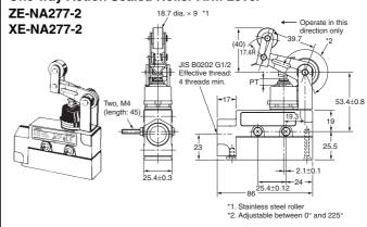
Note: 1. Unless otherwise specified, a tolerance of  $\pm 0.4$  mm applies to all dimensions.
