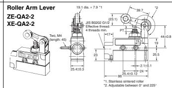
Note: 1. Unless otherwise specified, a tolerance of  $\pm 0.4$  mm applies to all dimensions.
