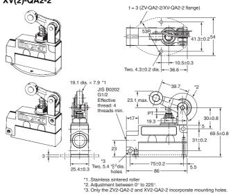
Note: Unless otherwise specified, a tolerance of  $\pm 0.4$  mm applies to all dimensions.
