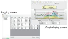
Insert the SD card containing collected data into a PC, and simply designate the drive in order to manage and graph the recorded data. Measurement data is stored in CSV format, allowing for easy temperature and humidity data management.
