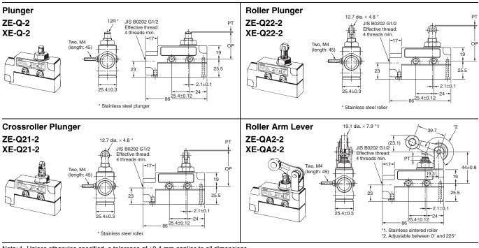
Note: 1. Unless otherwise specified, a tolerance of ±0.4 mm applies to all dimensions. 2. The diagrams shown the Switches with two, M4 screws (length: 45) attached. (The screws are provided.)
