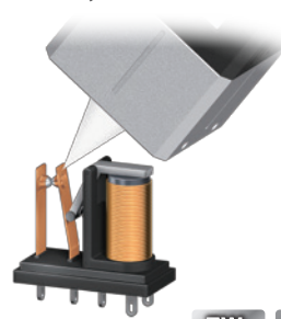
Operation inspection of relay contacts
