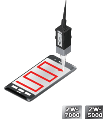
Flatness measurement of cover glass
