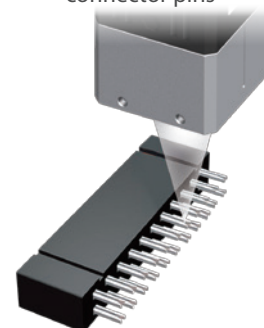
Coplanarity measurement of connector pins
