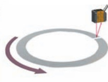
Checking welding point positions on ring gears
