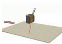
Inspecting the height of the core in cardboard
