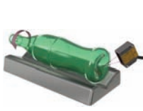
Detecting the indentation on glass bottles
