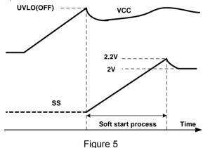
SS pin is also is used for external latch triggering (Please refer to "External Latch Triggering" section).
