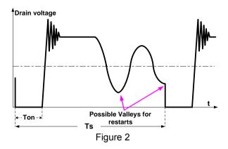
The typical detection level is fixed at 75mV at the DEM pin. Demagnetization is recognized by detection of a possible "valley" when the voltage at DEM is below 75mV in falling edge. DEM detection is suppressed during the ringing suppression time Tsupp (please refer to "Ringing Suppression Timer" section).
