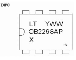
A:DIP8 Package; X: Version Num(X=C); P: Pb-free Package Y: Year Code(0-9) WW: Week Code(01-52) S: Internal Control Code(Optional)
