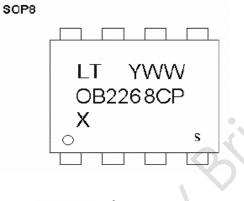
C: SOP8 Package; X: Version Num(X=C); P: Pb-free Package Y: Year Code(0-9) WW: Week Code(01-52) S: Internal Control Code(Optional)
