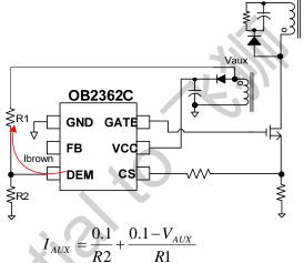
R1: The resistor connected from DEM to AUX.
