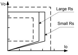
Fig.3 Adjustable output power by changing Rs
